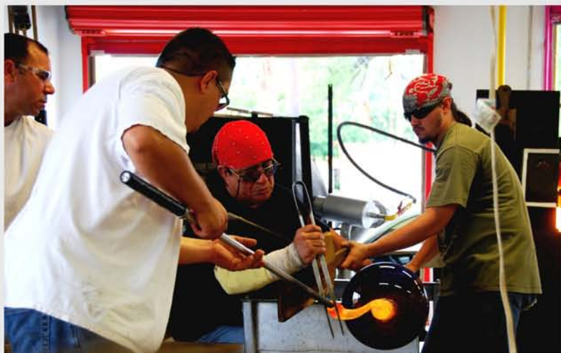
Adding a base to the glass
