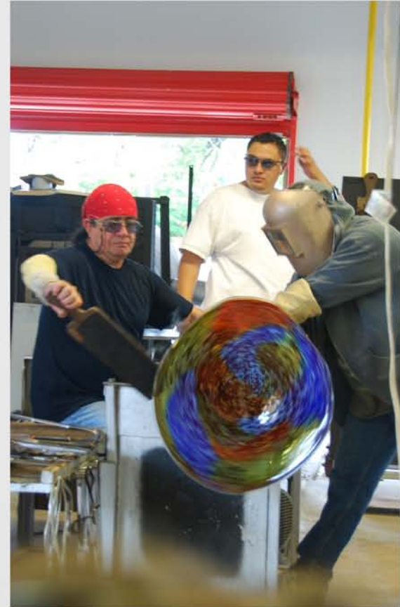
Final trimming of the plate
