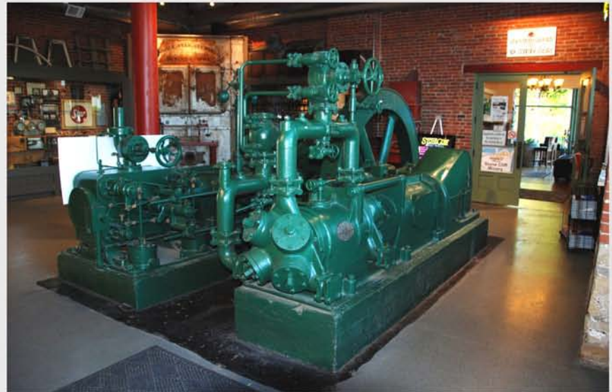
Old steam powered compressor - Star Brewery
