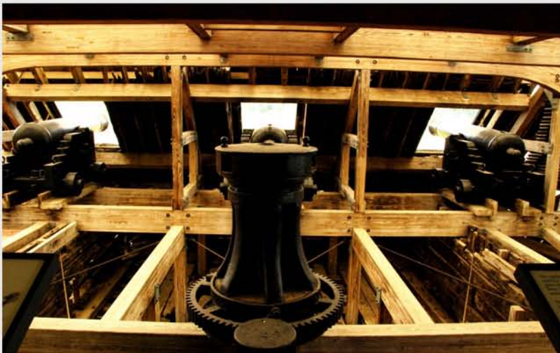
Capstan - steam driven winch for hauling the anchor and moving heavy guns
